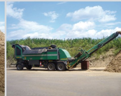
1600 XL-Version: With saddle chassis for easy road transport and with long feed chamber for maximum loading capacity.
