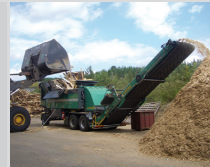
Attractive options for individual designs: Long conveyor belts; Magnet above the conveyor belt for sorting out metal; central lubrication system.
