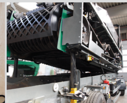
The chassis which can be lifted at the press of a button: Easy accessibility of the machine for extremely short hauls.
