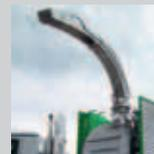
3 The material can be discharged via a slewable conveyor belt or a blower (only with LogChipper®).
