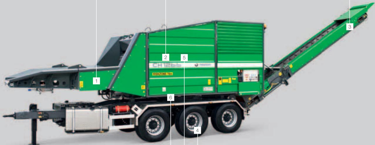
4 Mobility enhances the value: the machine can be moved via a 3-axle rigid drawbar trailer, mounted on a truck, as semi-trailer, or crawler-based.
